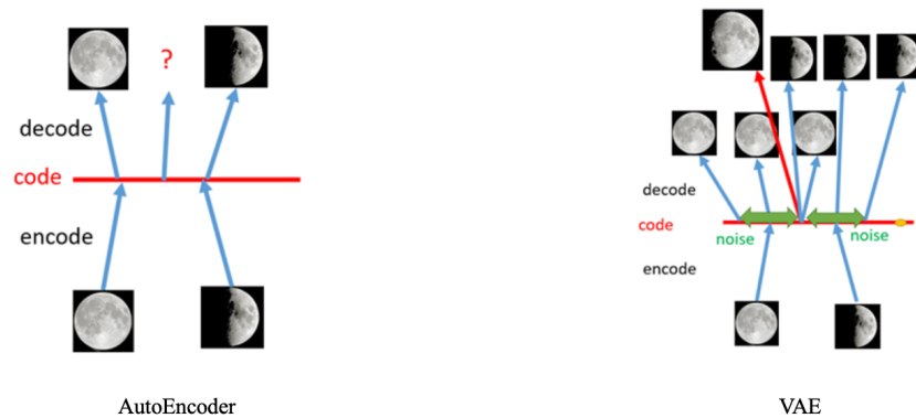
Figure 3 : The advantage of VAEs in generating more diverse and continuous data samples by incorporating noise into the latent space.
